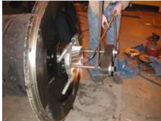
Figure 17. Heating the shell pinion
