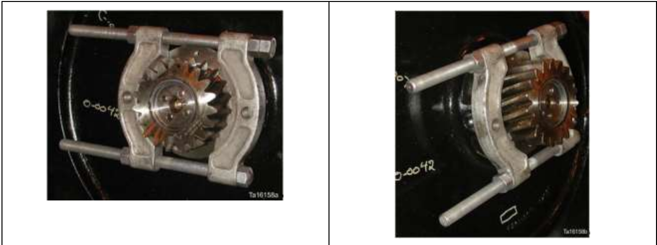
Figure 15. Bearing puller installation
